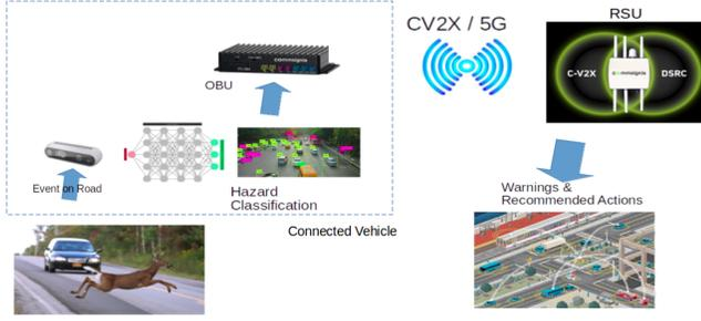
Fig. 1. Description of V2X leveraged hazard detection sensor.
