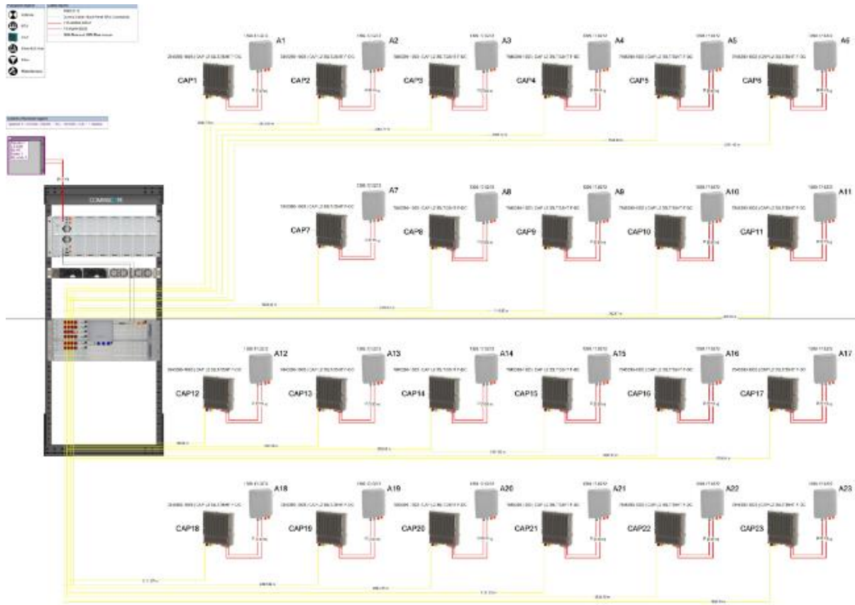
Figure 45: Detail 5G radio access Points connections to Master Unit
