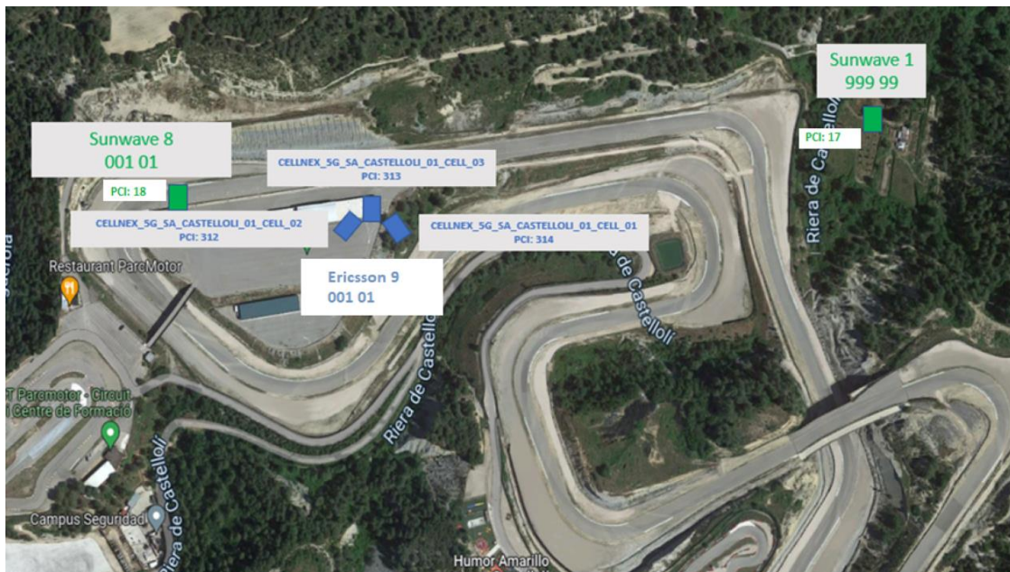
Figure 19: Location of gNodeBs and radio sectors in Castellolí test site.
