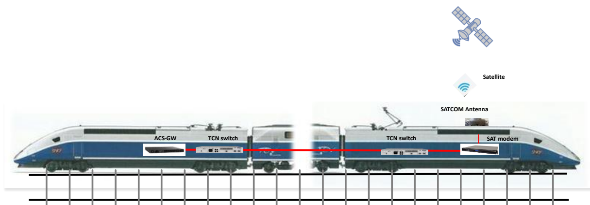
Figure 16 – On-board SAT radio access architecture.
