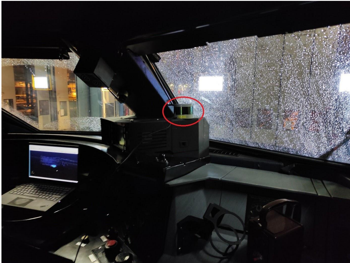
Figure 15 - Photograph of the LiDAR inside the TGV cockpit during the experiments
